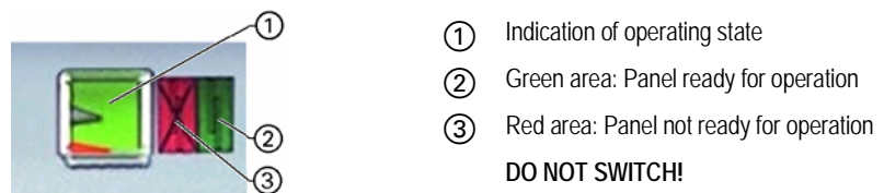
Fig. 69: Ready-for-service indicator for SF 6 gas (option)
