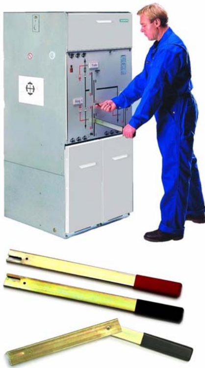
Fig. 29: Detachable lever with red handle for earthing and de-earthing, with black handle for load breaking / circuit breaking. Alternatives: One-lever operation and anti-reflex lever (reversing the switching direction requires re-inserting the operating lever)
