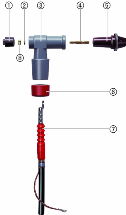
Fig. 21: Adapter for conventional cable sealing end
