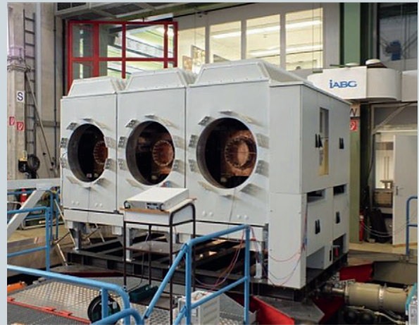
Fig. 54 HB3 switchgear during seismic testing
