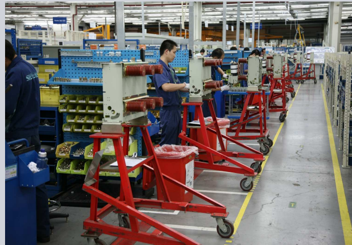
VCB assembly line
